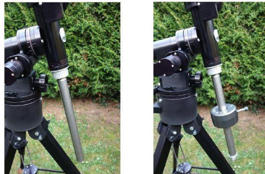
Screw the counterweight bar and install the counterweight
