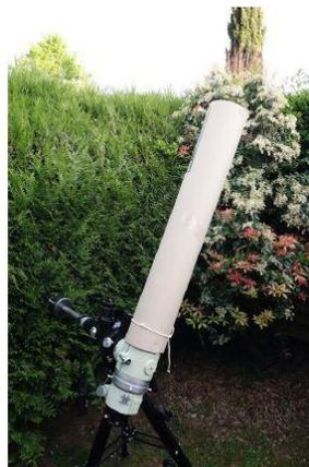
Cut cardboard, make a tube, insert it over the telescope shield and fix the ends.
