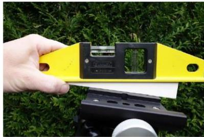
Use a bubble level and a triangle (cut according to the latitude) to adjust the latitude.
