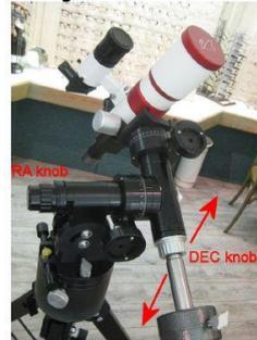
Unscrew RA knob, adjust counterweight balance.
