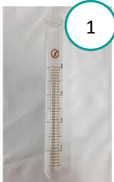
Tabung reaksi (berisi larutan \text{NaOH} , \text{HCl} , \text{CH}_3\text{COOH} , \text{NH}_4\text{OH} )
