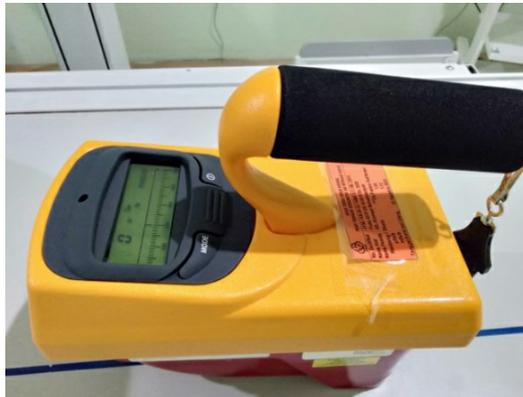
Gambar 2.6 Ion Chamber Surveymeter 451P
