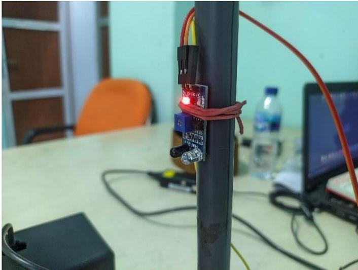
Gambar 0. 4 Proses Pengujian Sensor *Infrared Proximity* FC51
