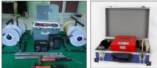
Gambar 3. 2 satu set geolistrik resistivity
