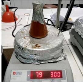
**Gambar 4. 12.** Proses pencucian biodiesel
