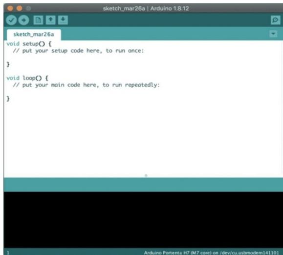
**Gambar 2.2:** Tampilan Interface Arduino IDE
