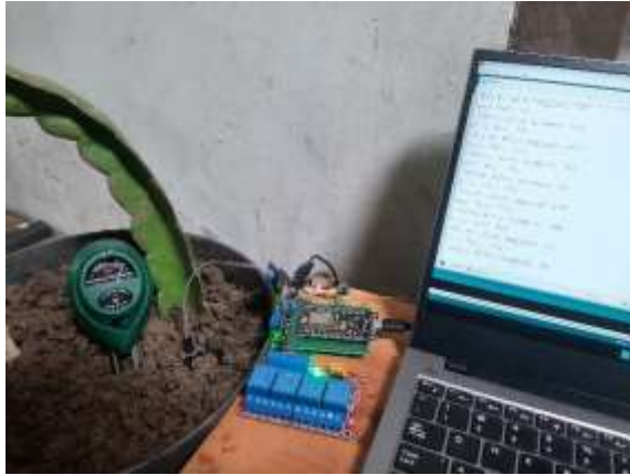
Gambar 4. 5 Pengujian soil moisture sensor
