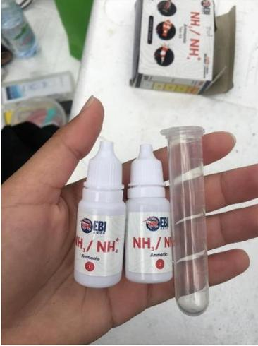
A photograph showing a hand holding two small white bottles of ammonia and a test tube. The bottles are labeled 'EBI' and 'NH <sub>3</sub> / NH <sub>4</sub> ' with 'Ammonia' written below. The test tube is clear and contains a small amount of liquid. In the background, there is a box of 'EBI' ammonia. | Teskit<br>ammonia                      |
