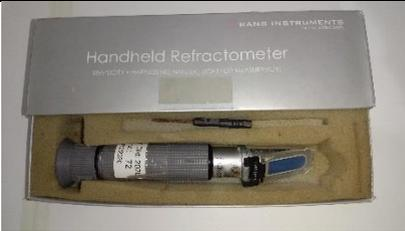
A handheld refractometer is shown inside its carrying case. The case is open, revealing the device which has a cylindrical body and a lens. The lid of the case is white and features the text "HAND INSTRUMENTS" at the top, "Handheld Refractometer" in the middle, and "SALINITY • REFRACTIVE INDEX • TEMPERATURE" at the bottom. The device is resting on a yellow foam insert. | Refraktometer |
