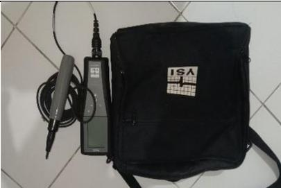
A DO meter is shown next to its carrying bag. The meter is a small, rectangular device with a digital display and a probe. The carrying bag is black and has a white label with the letters "ISA" on it. The entire setup is placed on a light-colored tiled floor.                                                                                                               | DO meter      |
