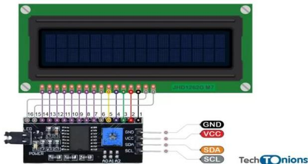
**Gambar 2. 4** Pin-Pin Modul LCD
