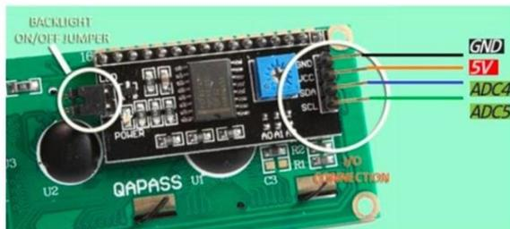
LCD display to Arduino wiring.
