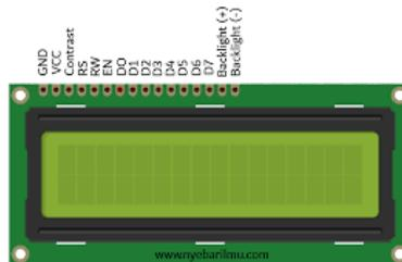
Gambar 2.7 LCD 16x2
