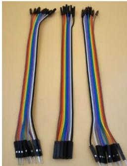
Gambar 3.7 Kabel Jumper
