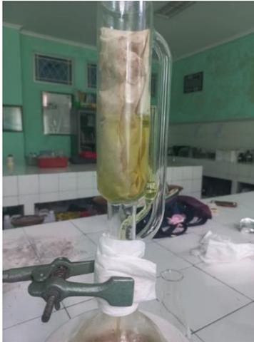
**Gambar 4. 3** Ekstraksi Soxhlet Biji Nyamplung
