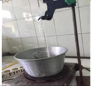
A water bath setup. A metal pot is placed on a stove, and water is being poured from a blue container into it. A metal stand is visible in the background.     | <p>Proses pemanasan ekstrak menggunakan waterbath agar mendapatkan ekstrak kental</p> |
