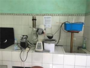
A laboratory setup for evaporation. A blue container is mounted on a stand, with a tube leading to a beaker. A white container is also visible on the counter. | <p>Proses evaporasi hasil maserasi</p>                                                |
