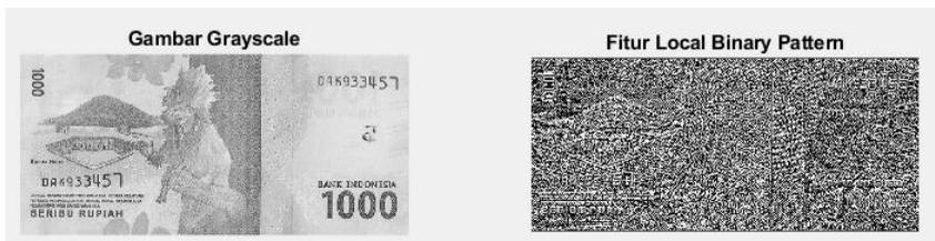
Gambar 3. 5 Grayscale ke Local Binary Pattern
