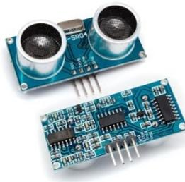
Gambar 2.6 Sensor Ultrasonik HC-SR04
