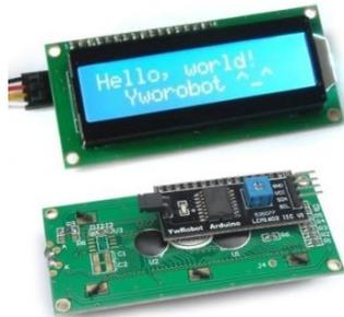
Gambar 2.8 Modul LCD I2C
