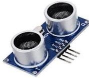
Gambar 2.1 Sensor Ultrasonik HC-SR04
