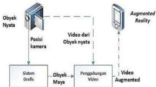
Gambar 2.4 Diagram Kerja *Augmented Reality*
