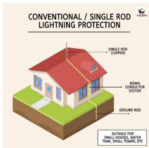
Gambar 51 Penangkal Petir Sistem Franklin
