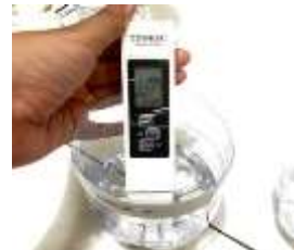
Gambar 4.4 Pengujian TDS Meter air sumur x
