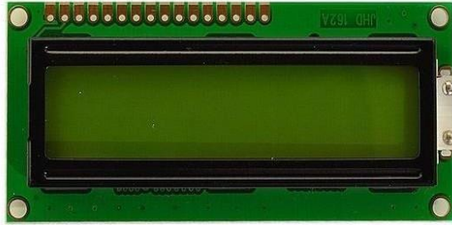
Gambar 2. 7 Modul LCD I2C
