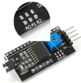
Address selection pads in the I2C-to-LCD piggy-back board.
