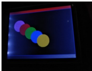
Tampilan Filled Circle modul LCD
