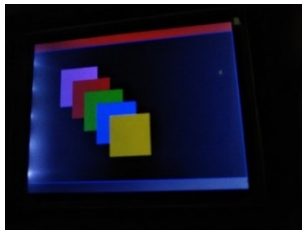
Tampilan Filled Rectangle modul LCD
