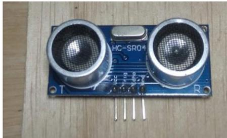
Gambar 2. 1 Sensor ultrasonik/Sensor Ultrasonic
