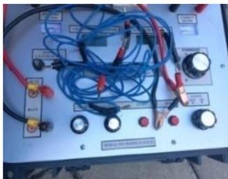
**Gambar 3.2 Alat Resistivitymeter**
