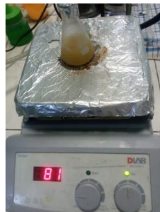
Proses pencucian biodiesel
