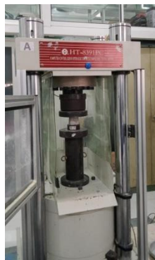
Gambar 2.7 Alat Uji Kuat Tekan ( Compression Testing Machine )
