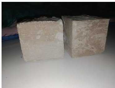
Gambar 4.4 Paving Block 100% Semen
