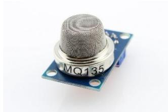
*Gambar 2.3 Sensor karbon CO<sub>2</sub>*
