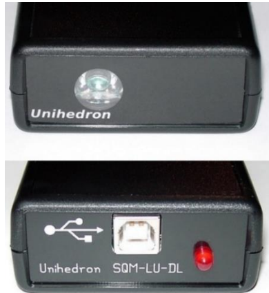
Gambar 3. 2 SQM LU - DL (Lens USB Data Logger) 99
