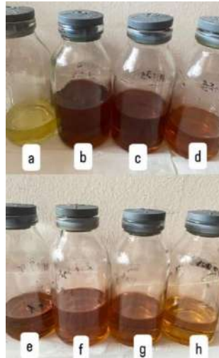
Gambar 4. 5 a). Minyak Goreng Baru, (b). Minyak Jelantah (MJ), (c). MJ + HFKS 3 g, (d). MJ + HFKS 5 g, (e). MJ + HFKS 7 g, (f). MJ + HFKS \text{H}_3\text{PO}_4 10% 3 g, (g). MJ+ HFKS \text{H}_3\text{PO}_4 10% 5 g, (h). MJ + H FKS \text{H}_3\text{PO}_4 10% 7 g
