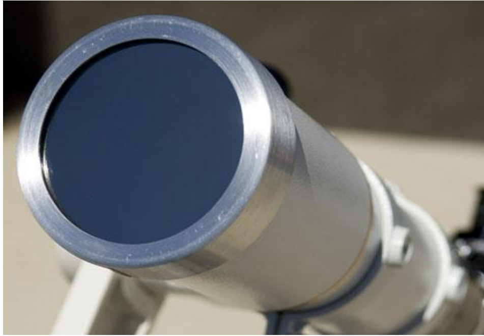
Gambar 3: Filter : Thousand Oaks Optical Solar Filters RG 3750 for Megrez 72 3
